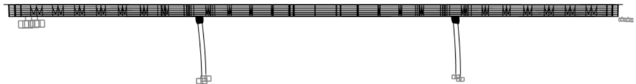
Figure 2.32. Mode 1 of vibration (longitudinal translation), T_1=2.14s , f_1=0.47 Hz
