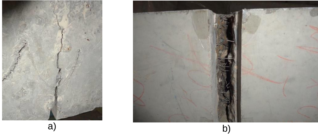
Fig. 1. The failure mode of the specimen. Side view (a) and bottom view (b).
