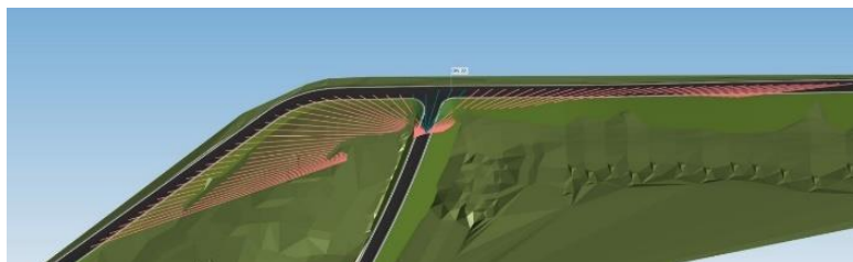
Figure 84. Sight distance perspective for 1:4 slope
