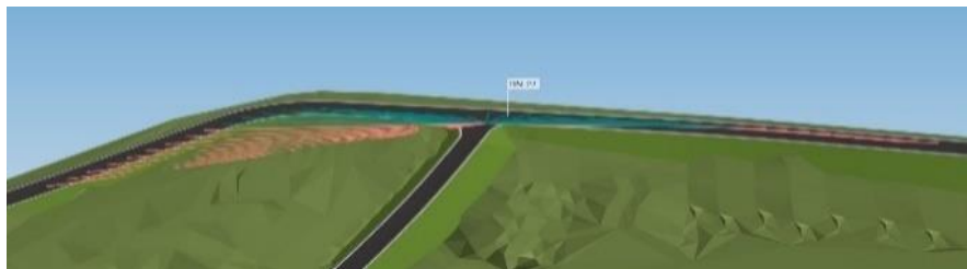
Figure 76. Sight distance perspective for 1:4 slope
