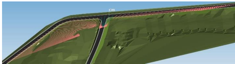
Figure 82. Sight distance perspective for 1:2 slope
