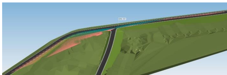
Figure 72. Sight distance perspective for 1:4 slope
