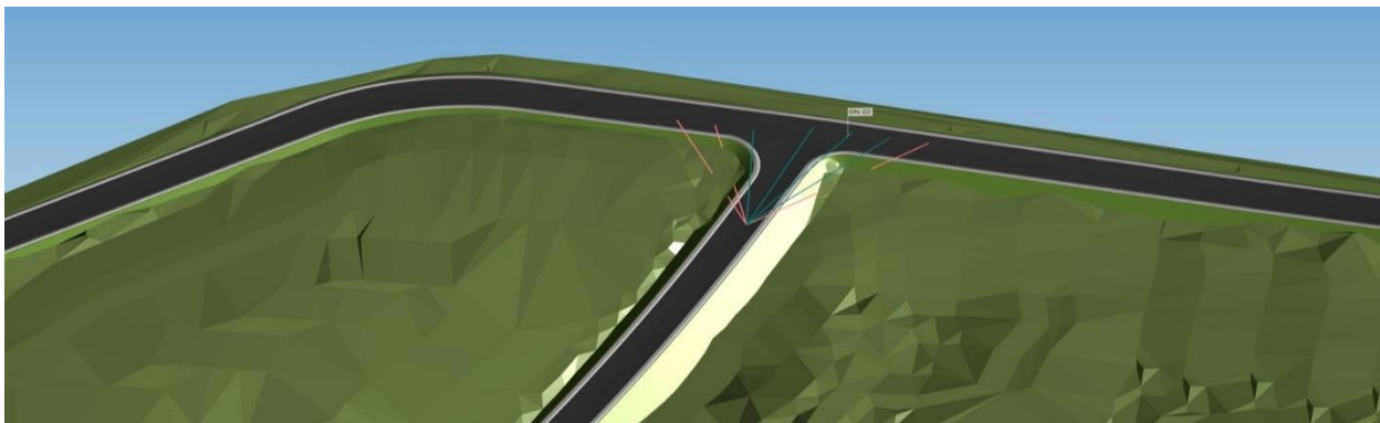
Figure 93. Sight distance perspective for a 1:2 side slope
