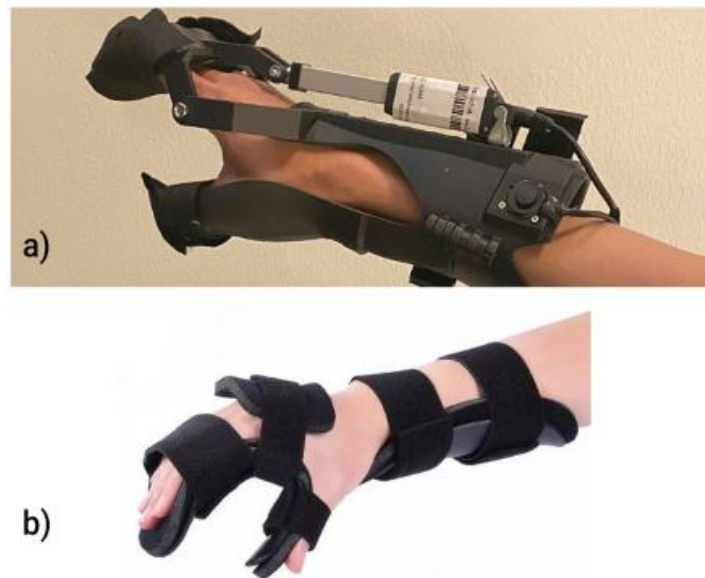
Figure 13. Comparison between two types of orthoses: (a) customized hybrid orthosis NuroSleeve, with active control and integrated stimulation [92]; (b) classic passive wrist orthosis [93].
