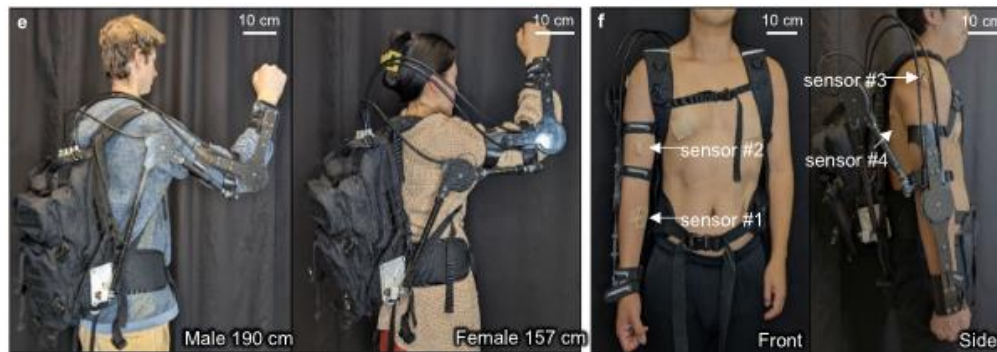
Figure 8. Upper-limb exoskeleton equipped with deformable sensors, designed to adjust the level of assistance according to the patient's movements and effort [72].
