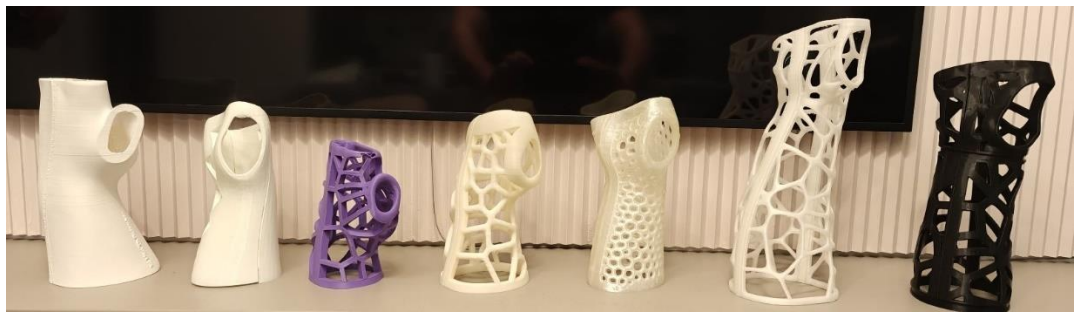
Figure 19. Various orthosis models manufactured through 3D printing [99]
