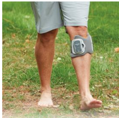
Figure 7. The Bioness L300 Go device used for functional electrical stimulation of the dorsiflexor muscles during walking [61]
