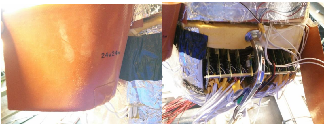
Fig. 2 – A mounted patch (24V, 24W) and the acquisition boards of Thermal Boy
