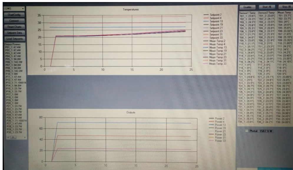
Fig. 3 – Graphical interface of Thermal Boy, power and temperature of every patch
