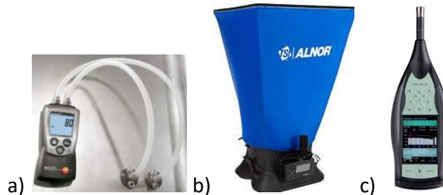
Fig. 26– a) Testo differential pressure gauge for filter pressure loss; b) TSI balometer type ALNOR; c) Bruel & Kjaer sound meter
