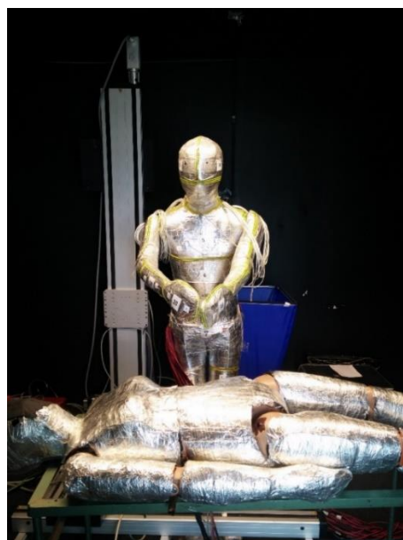
Fig. 41– Suzy and Thermal Boy as a patient and a surgeon in the climatic chamber
