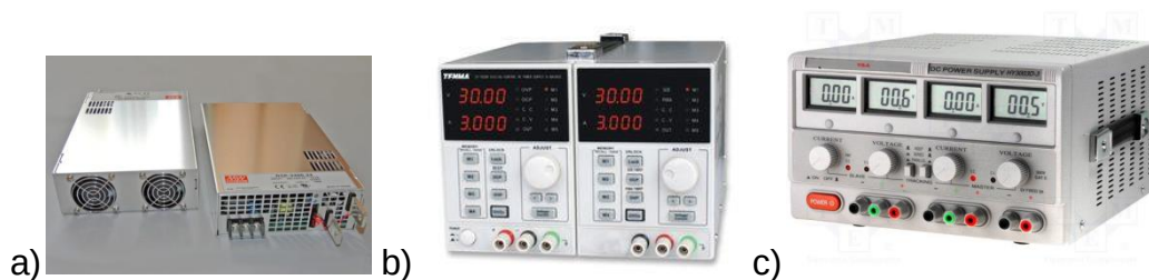
Fig. 12– Power sources for: a) patches; b) temperature controller; c) temperature acquisition
