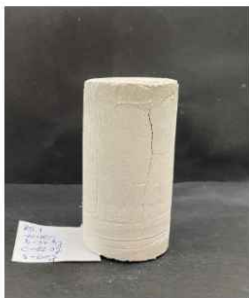
Fig. 2.5: Samples affected by cracking
