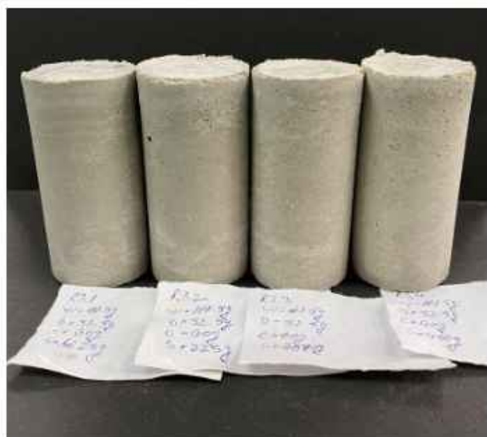
Fig. 2.3: The aspect of a group of samples with the same water-cement-bentonite ratio after removing the cast
