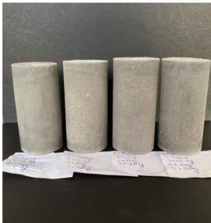
Fig. 2.4: The aspect of a group of samples with the same water-cement-bentonite ratio after removing the cast
