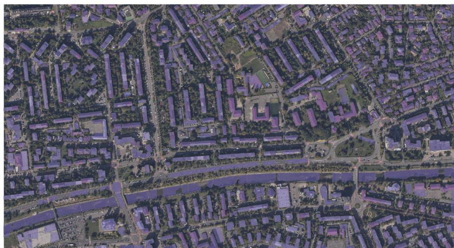
Figure 5.25. Buildings Footprints Generated with the Trained DL Model
