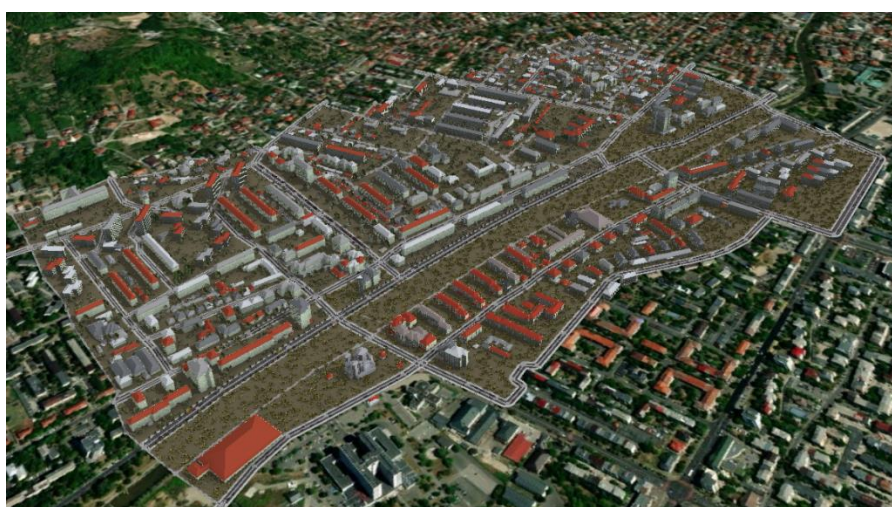
Figure 5.42. Area modelling in CityEngine with LOD detail level 3 (LOD3.1, According to the Classification Made by Biljecki et al. (2016)), Overview
