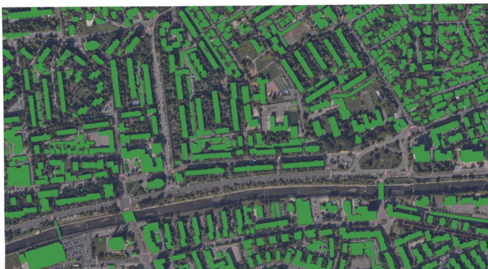
Figure 5.28. Buildings Footprints Generated from the LiDAR Point Cloud
