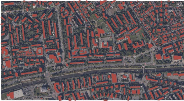
Figure 5.23. The Results of Extracting Buildings Footprints with the DL Model in ArcGIS Living Atlas
