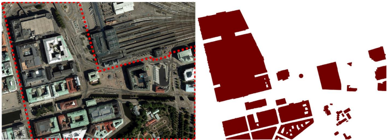
Figure 3.3. Classification of an Image (left side) by SVM Algorithm, Obtaining the Buildings Footprints (right side) (Aslani & Seipel, 2020)
