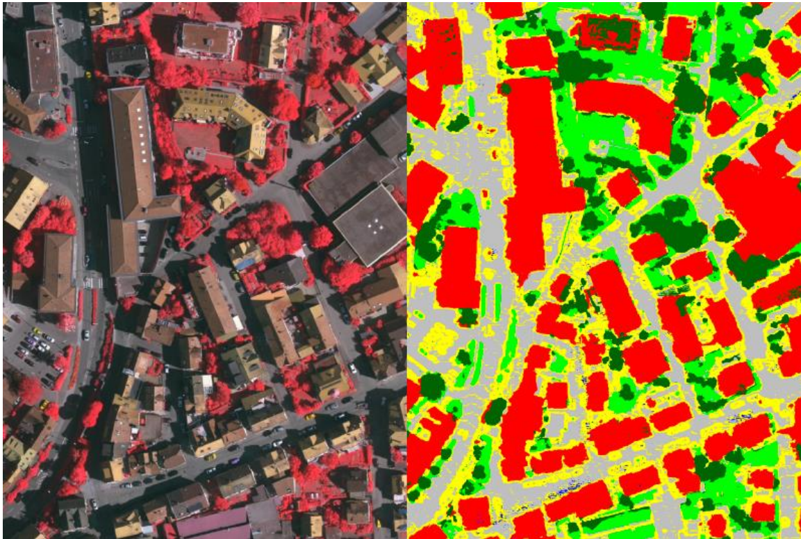
Figure 3.1. Orthorectified Image (left) and Image Classification Result (right): red-construction, dark green-tree, light green-low vegetation, grey-waterproof surface, yellow-cars (Höhle, 2017)
