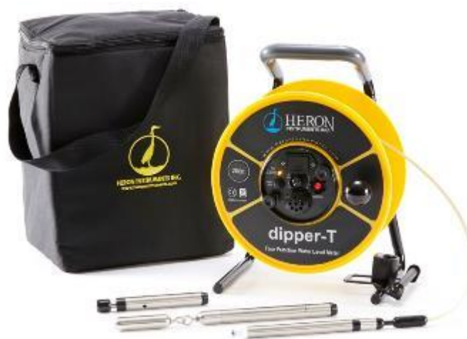
Figure II.3 - Groundwater level monitoring equipment
