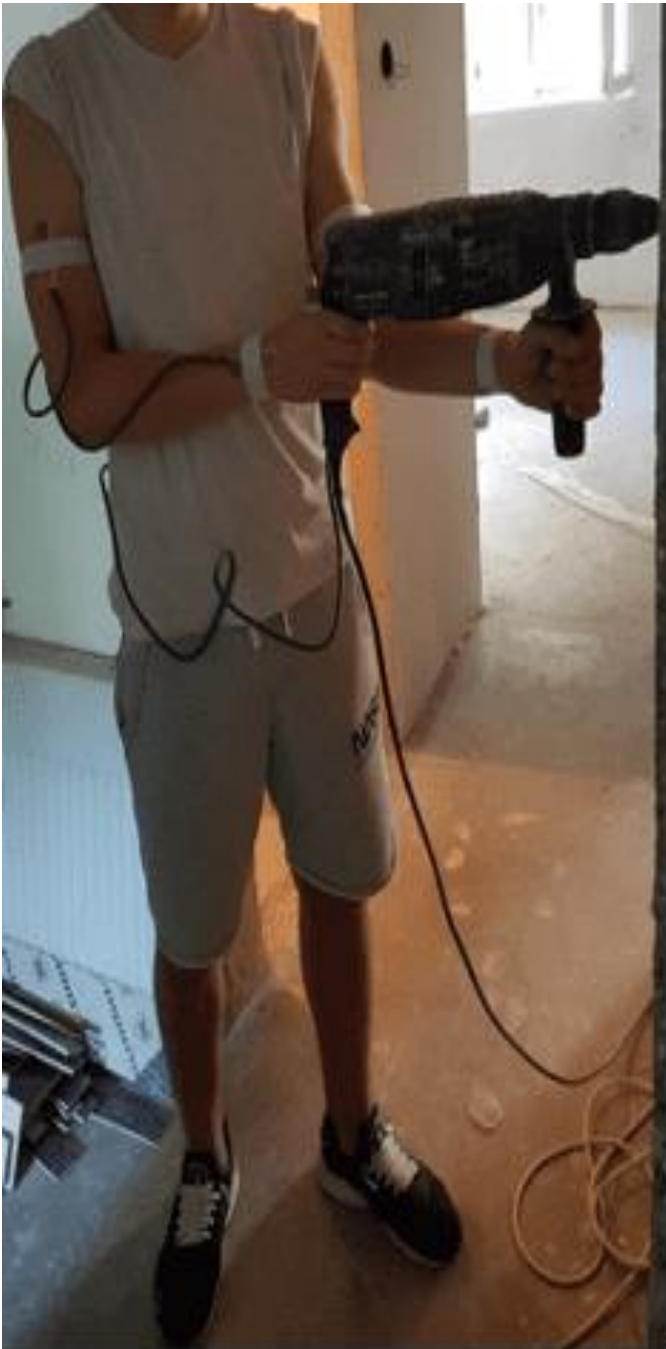
Fig. 4.10. Mounted system for data collection drill with percussion - front view
