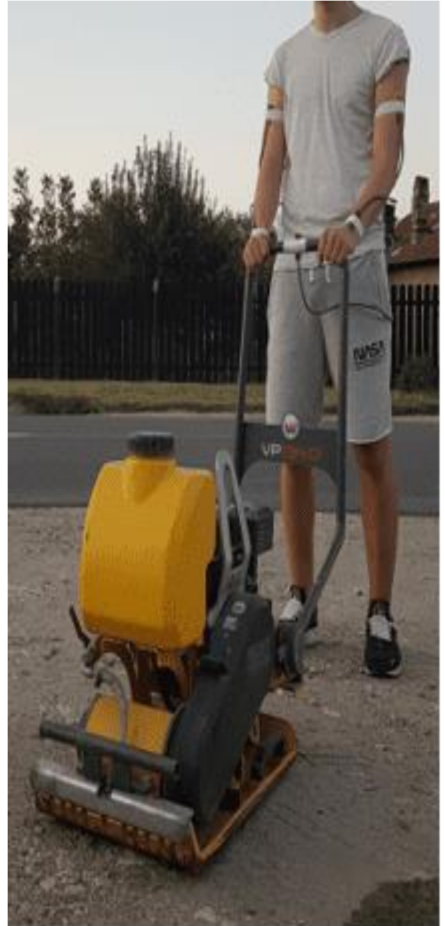
Fig. 4.17. Mounted vibrating plate data collection system - side view
