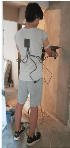
Fig. 5.5. Purchase system mounted for percussion drill data collection - side view
