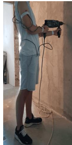
Fig. 5.6. Purchase system mounted for percussion drill data collection - side view
