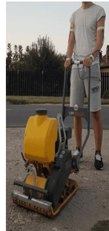
Fig. 5.11. Mounting system mounted for vibrating plate data collection - side view
