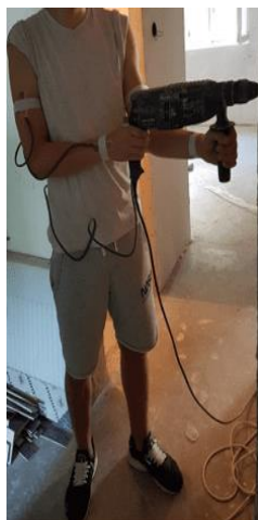
Fig. 5.7. Purchase system mounted for percussion drill data collection - front view
