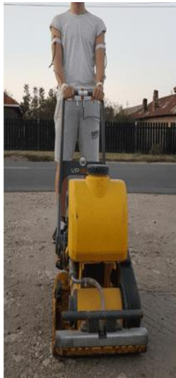
Fig. 5.10. Mounting system mounted for vibrating plate data collection - front view
