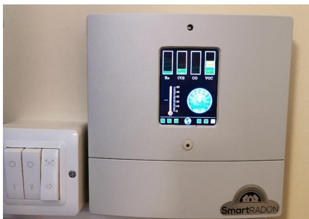
Figure 3 – Prototype equipment for continuous radon measurement SMART_RAD_EN
