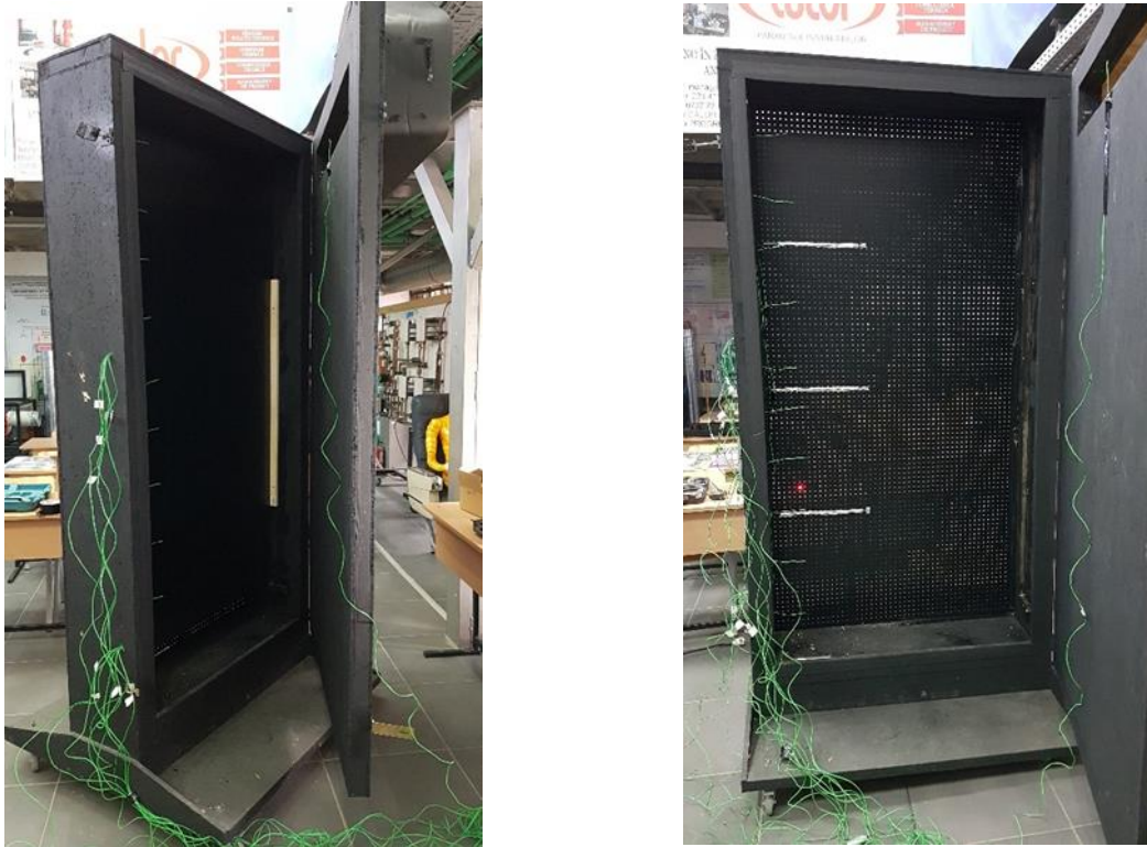
Figure 20. Thermocouple distribution for the DSTSC (left) and TSC (right)
