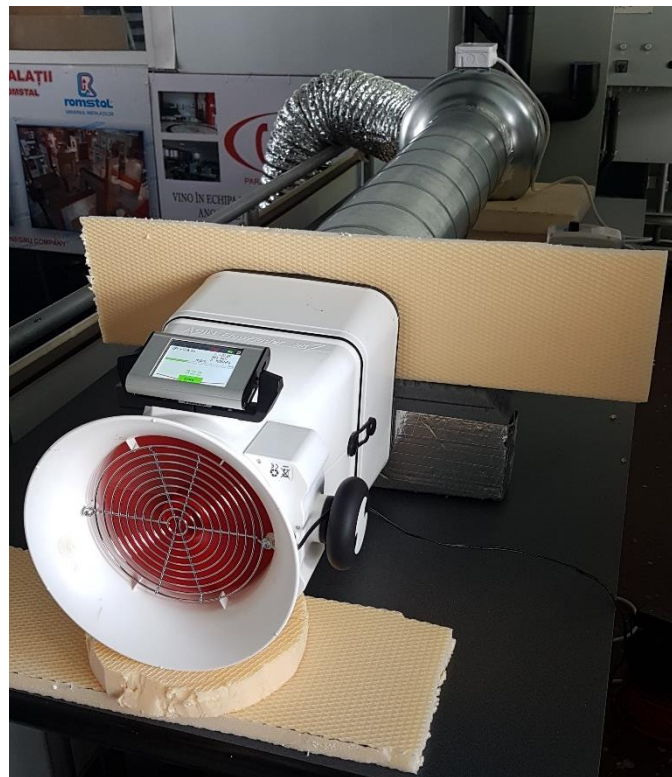
Figure 7. Utilization of the flow meter during an indoor experiment
