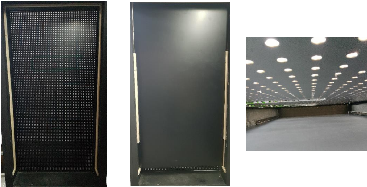
Figure 4. Interior view of the DSTSC, without back-pass, with back-pass and front air gap, from left to right.
