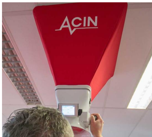
Figure 8. The FlowFinder®mk2 used on false ceiling for air flow measurement
