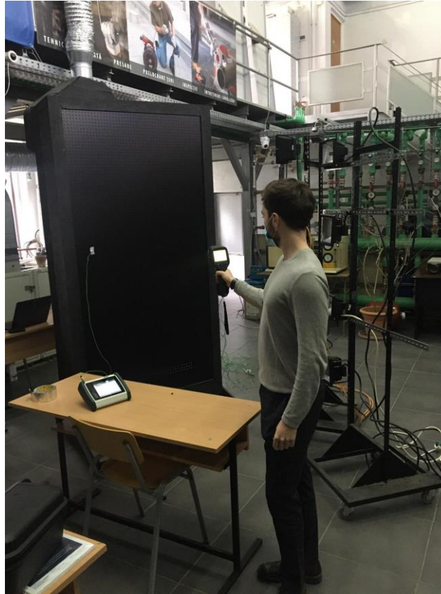
Figure 9. Measurement of the emissivity of the absorber plate using IR camera and thermocouples.
