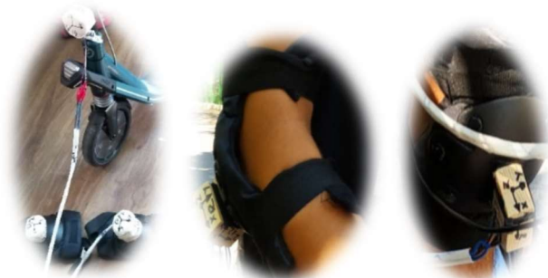
Figure 23 Scooter, elbow rest, knee brace with accelerometers
