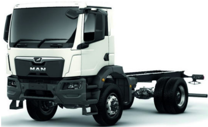
Fig. 25 (Figure 5.38): MAN TGM 18.320 motor truck with 4x4 drive.
