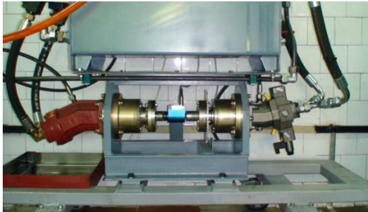
Fig. 6 EP2 type Bosch servomotor in the secondary side of the hydrostatic transmission (right), coupled to the hydraulic load simulation device.
