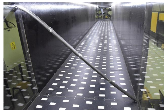
Figure III-4 – Scale model (tensioned cable)
