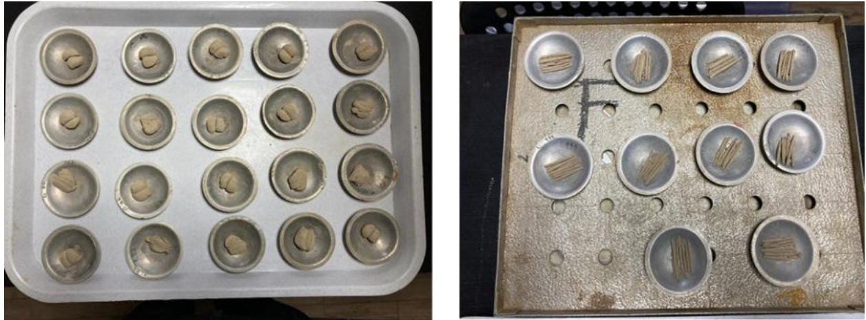
Fig. 39. Atterberg limits tests for non-treated and treated soil with different percentage of Nano-MgO a) Liquid limit test b) Plastic limit test
