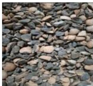
Figura 3.5. Material filtrant – granule ceramice.
