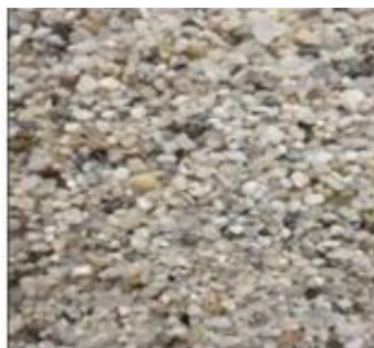
Figure 3.4. Filter material - filter sand.
