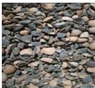
Figure 3.5. Filter material - ceramic granules.
