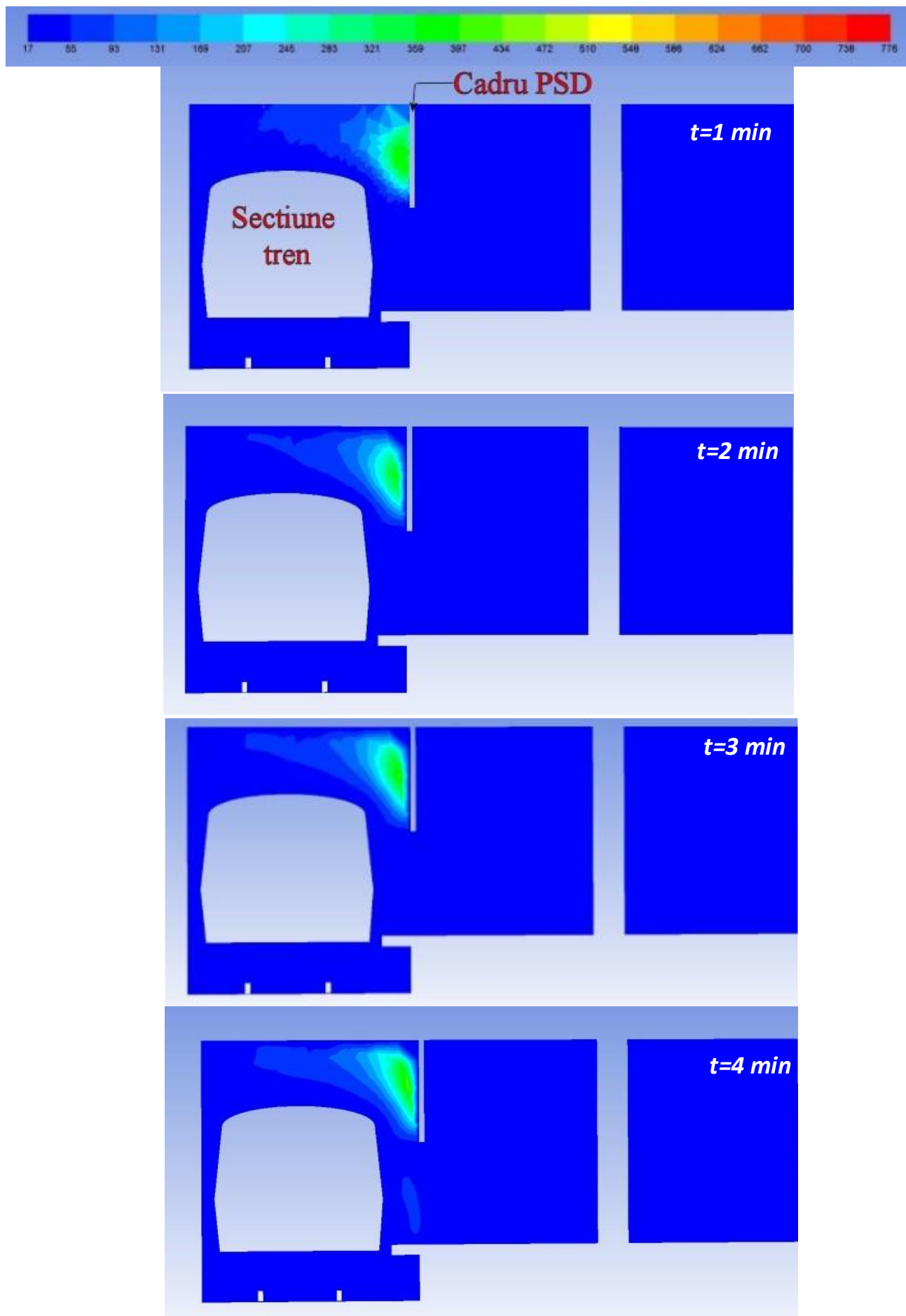
Fig. 33 Cross-section through the PSD door near the fire – air temperature fields - minutes 1-4 ( ^{\circ}\text{C} )
