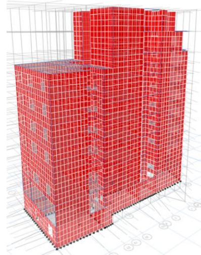
Fig. 13.2.3. 3D numerical model for the modelling variant that involves “shell” walls
