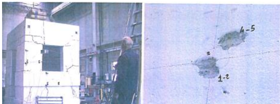
Fig. 6.2.2. The footprint of the 5 shocks within the second contact point [23]
