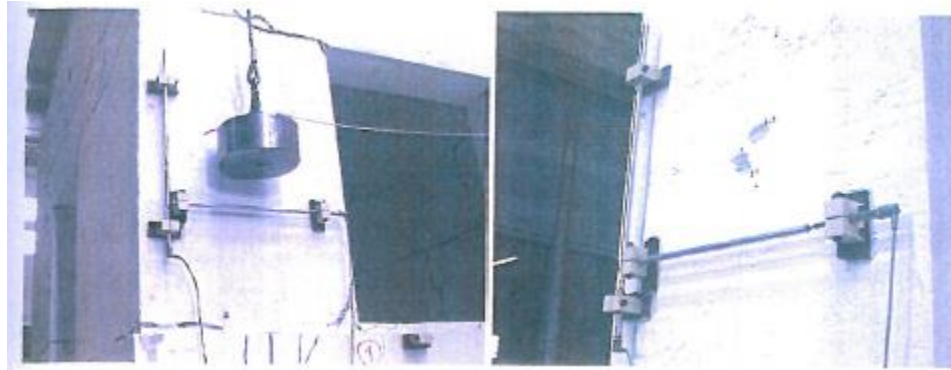
Fig. 6.1.2. The second contact point on the coating of the wall in an area without cracks [23]
