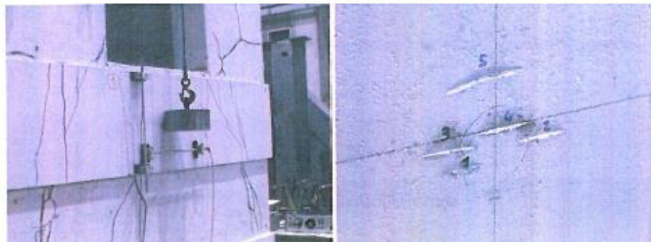
Fig. 6.2.1. The footprint of the 5 shocks within the first contact point [23]
