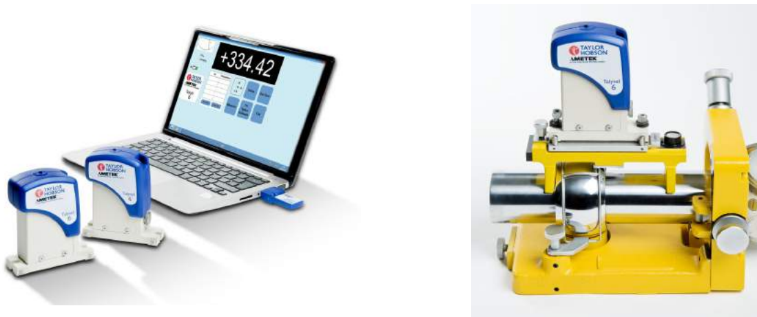
Figure 3.22 Talyvel electronic level (Taylor Hobson). [21]
