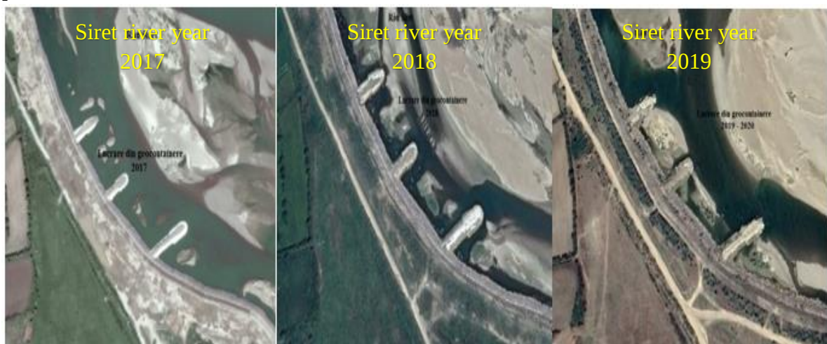
Fig.9.12. Vegetation development on geocontainer works
