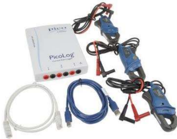
Figure 48 Experimental study bench current clamps and data acquisition station
