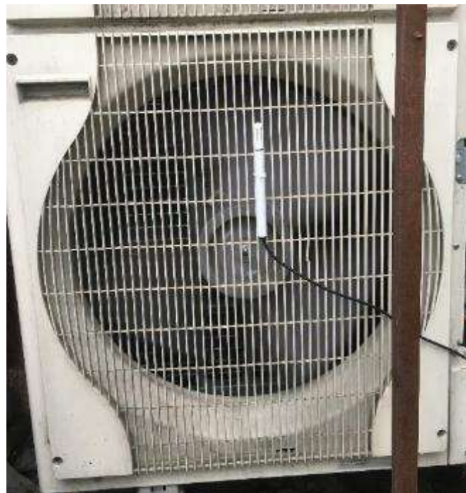
Figure 54 Experimental study bench evaporator output air temperature sensor location
