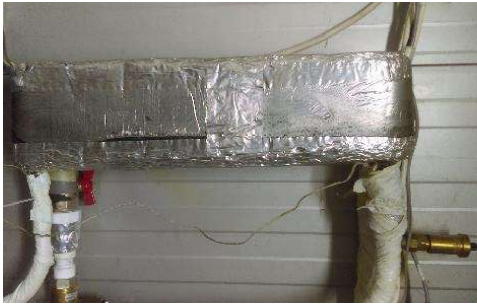
Figure 45 Experimental study bench heat plate exchanger condenser
