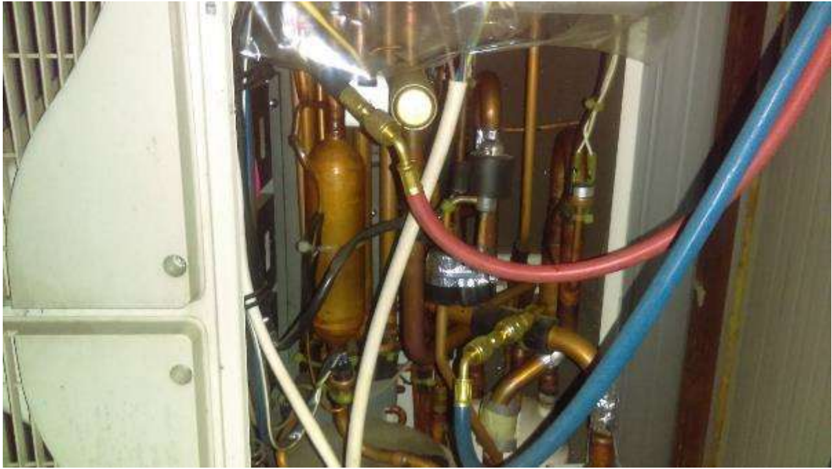
Figure 57 Experimental study bench cold and hot gas lines pressure measurement plugs
