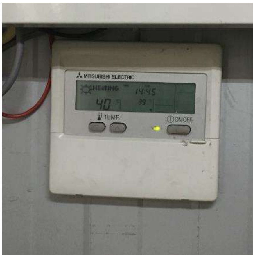
Figure 44 Experimental study bench heating temperature remote control
