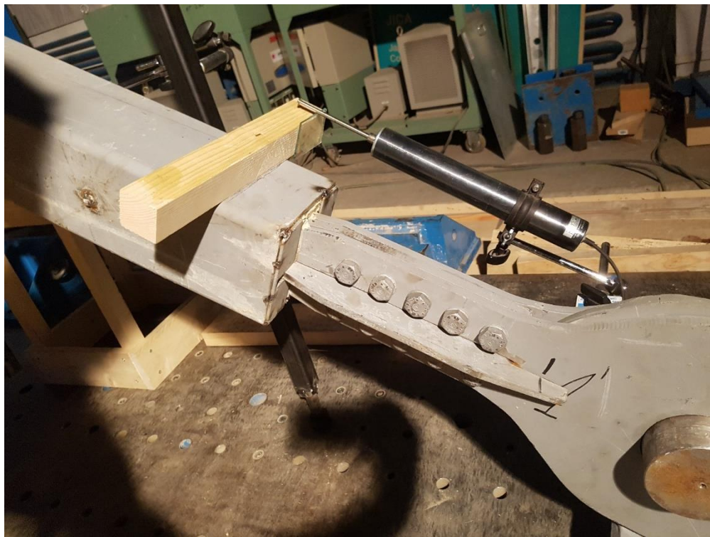
Fig. 5.9 – Assembly of transducer no.4
