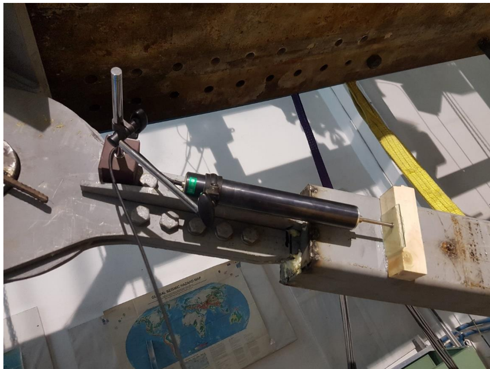
Fig. 5.7 – Assembly of transducer no.3
