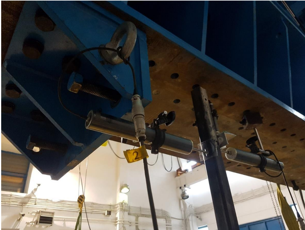
Fig. 5.6 – Assembly of transducers no. 1, no. 2 and no. 5
