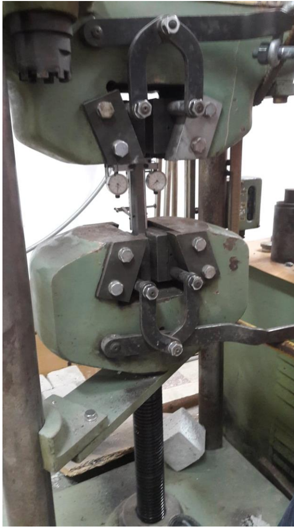
Fig. 6.3 – Tensile testing of standardized specimens
