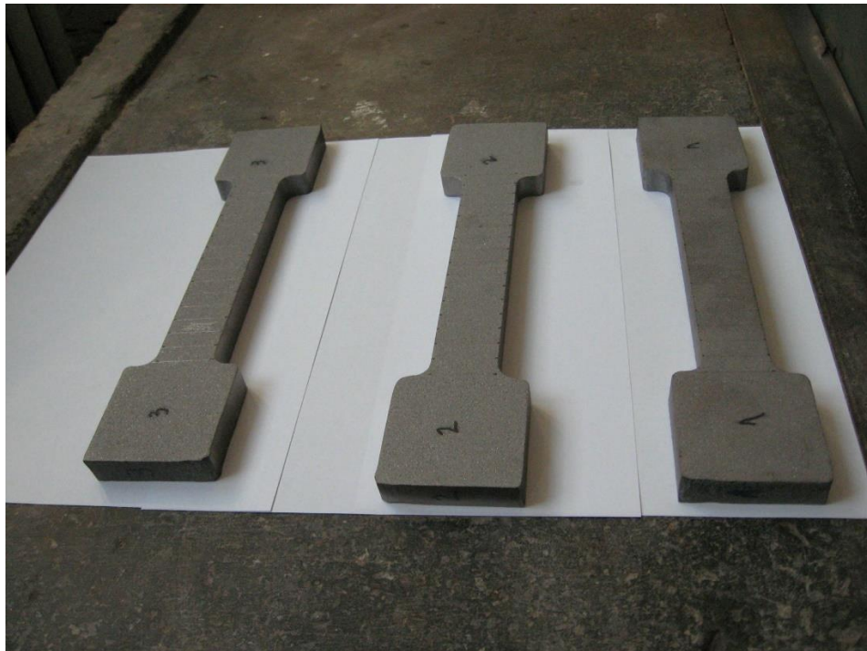
Fig. 6.4 – Marking of parts on test specimens for tensile testing
