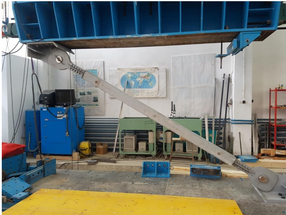
Fig. 3.9 – Mounting in the test position of the BRB prototype
