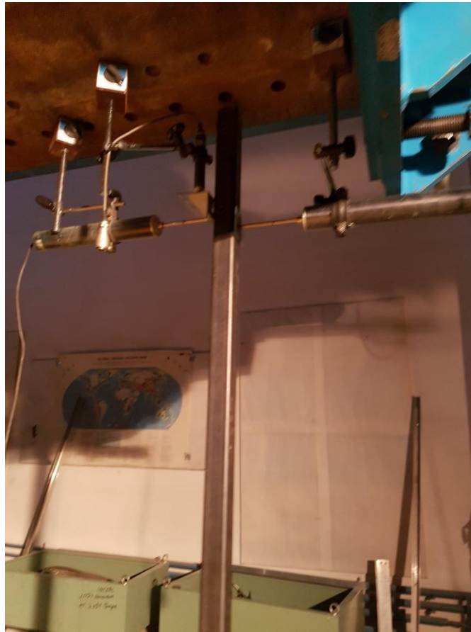
Fig. 5.10 – Assembly of transducers no.1, no.2 and no. 5
