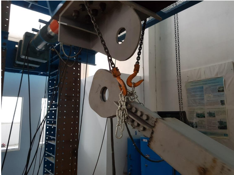
Fig. 3.8 – Mounting in the test position of the BRB prototype
