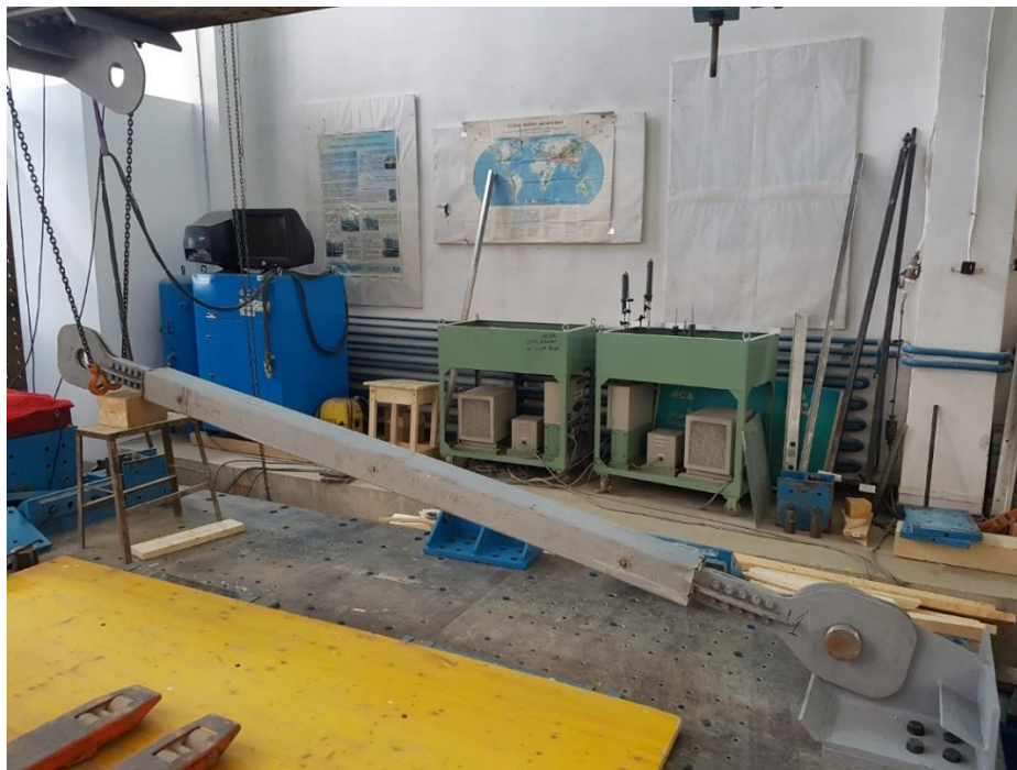
Fig. 3.7 – Mounting in the test position of the BRB prototype
