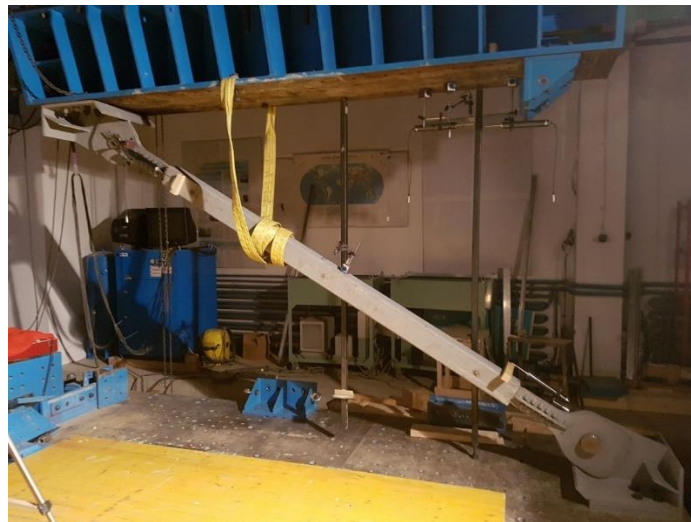
Fig. 5.1 – Assembly of transducers for the BRB prototype
