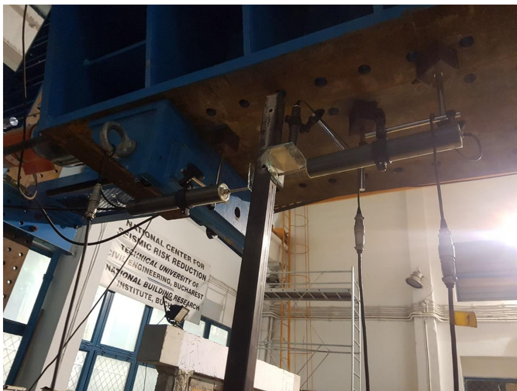
Fig. 5.5 – Assembly of transducers no.1, no.2 and no.5
