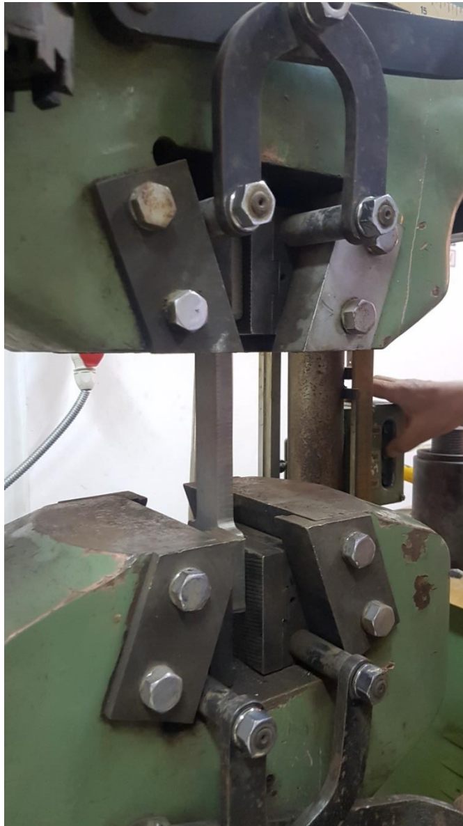
Fig. 6.2 – Tensile testing of standardized specimens
