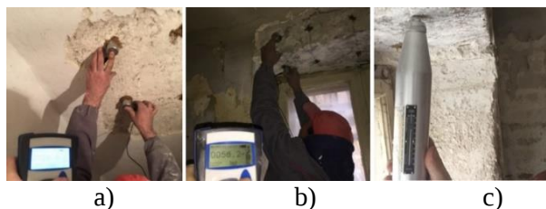
Figure 6.28 - Specimens (RC-1; RC-2; RC-3) subjected to non-destructive (determination of bulk density) and destructive (determination of standardized compressive strength) laboratory tests [122]
