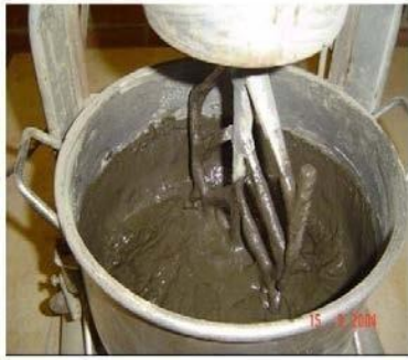
Figure 1 Fresh Geopolymer Binder Paste [4]
