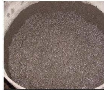
Figure 2 Fresh Geopolymer Concrete [4]
