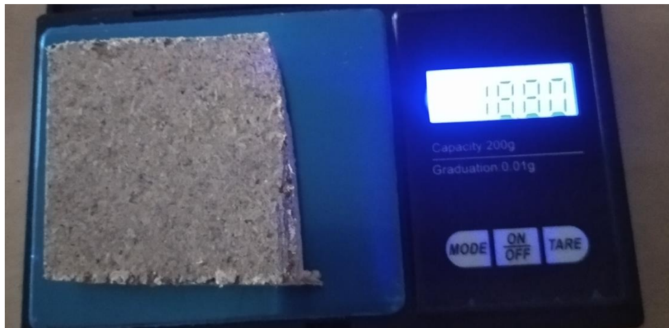
Fig 19. Particle board sample weighing before testing
