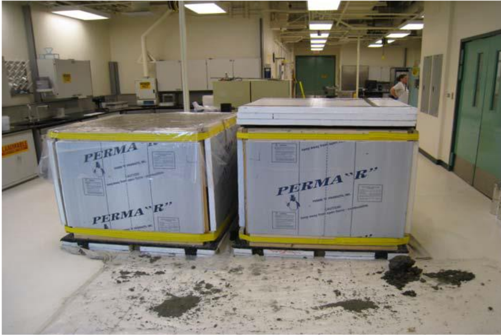
Figure 27 Uninsulated (left) and insulated (right) mass concrete block specimens
