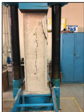
a) Concrete column (CP-Cnt1)
