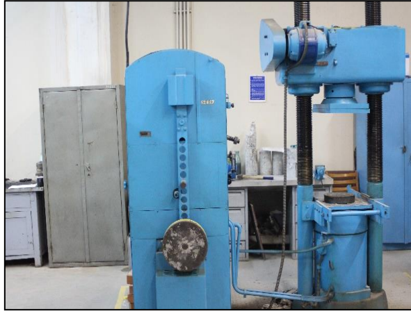
Fig. 3-4: Universal testing machine used to test concrete columns.
