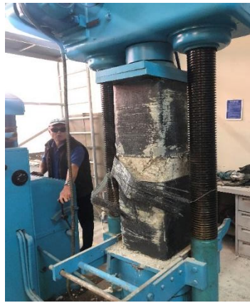
Fig. 4-2 b: Failure mode of the strengthened column (CP-4).
