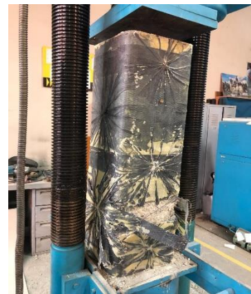
Fig. 4-2 c: Failure mode of the strengthened column (CP-5).
