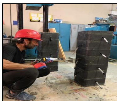
e) Inject Mapefix VE SF 300 fastener to fill the holes.
