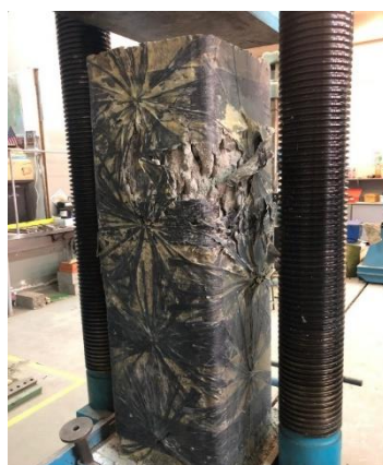
Fig. 4-3 e: Failure mode of the strengthened column (CP-7).
