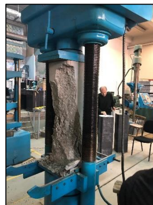
b) Concrete column (CP-Cnt2)
