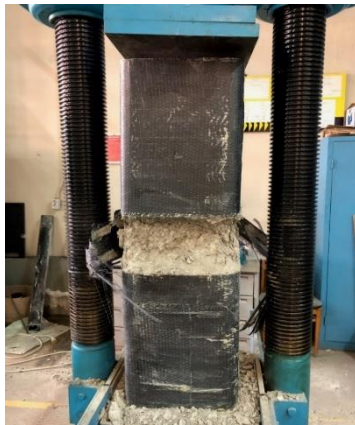
Fig. 4-2 a: Failure mode of the strengthened column (CP-3).
