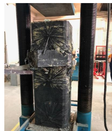
Fig. 4-3 f: Failure mode of the strengthened column (CP-8).
