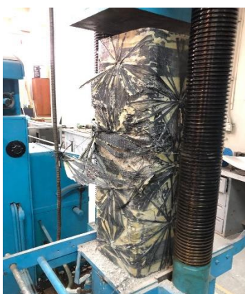
Fig. 4-2 d: Failure mode of the strengthened column (CP-6).
