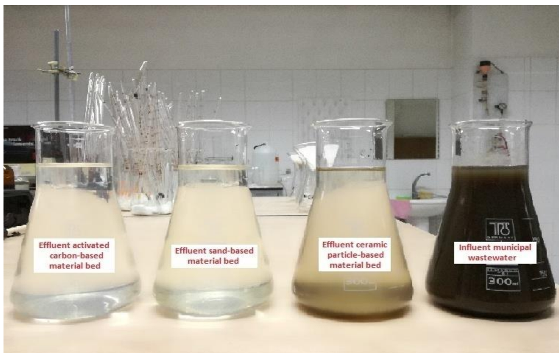
Figure 4.3. View of the effluent from the activated carbon-based filtration media bed, sand-based filtration media bed, and ceramic particle-based filtration media compared with the influent municipal wastewater.
