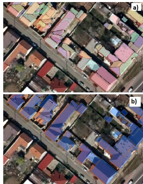
Figure 6.7 Buildings footprints a) segmentation results ; b) postprocessing results
