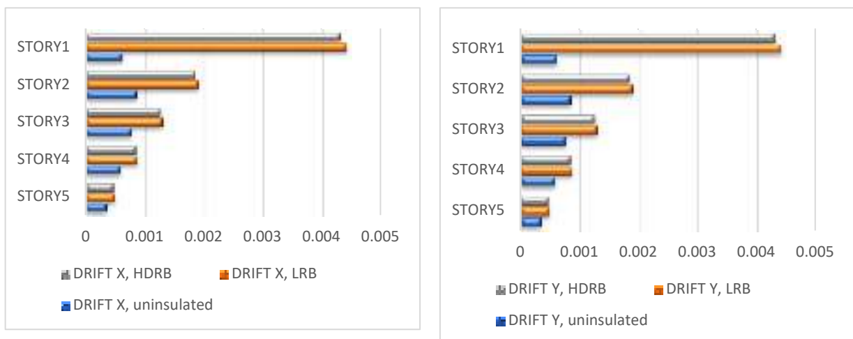
Figure - 37 Relative displacements for square buildings with UG+GF+4L on x and y directions
