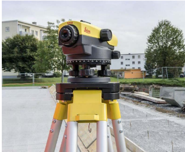
Figure 7. Optical level for checking the stability of the reference beams
