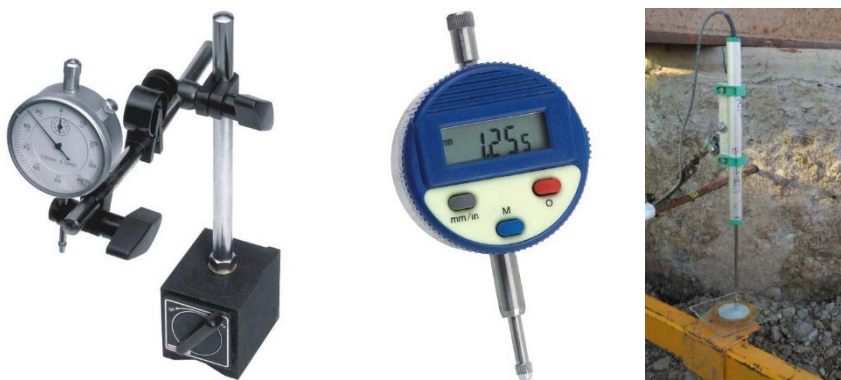
Figure 6. Dial gauge with magnetic installation system and analog clock (left), with digital display (middle) and electronic transducer (right)
