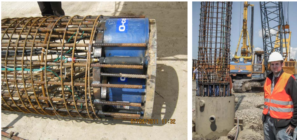
Figure 4. O-Cell hydraulic cells for Osterberg type test for LT2 (left) and LT1 (right) tests
