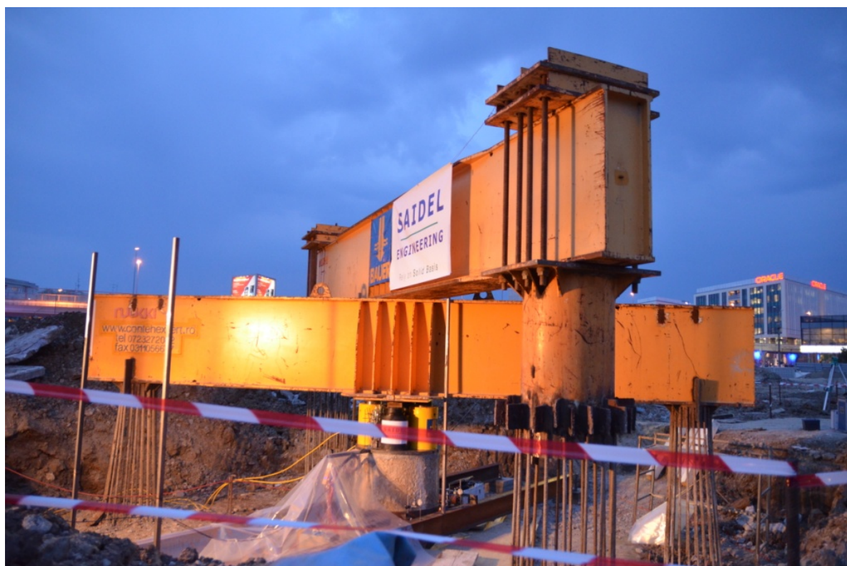
Figure 4. Axial compression test overview
