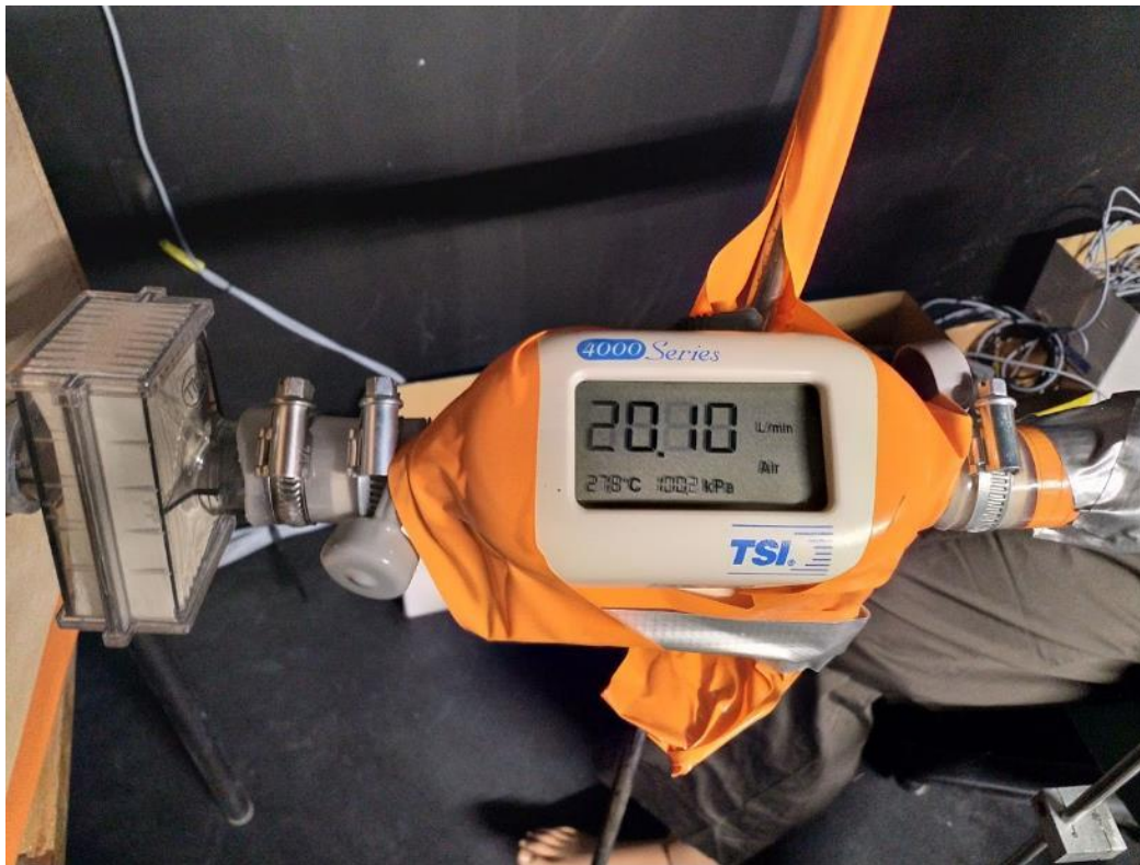
Figure 41 The TSI flowmeter during the measurements.
