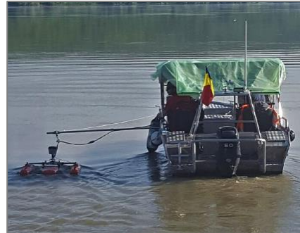
Figure 14. Towing the ADCP systems during measurements Tractarea
