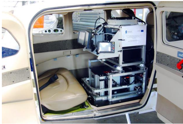
Figure 7. LiteMapper 6800i LiDAR system installed in the plane
