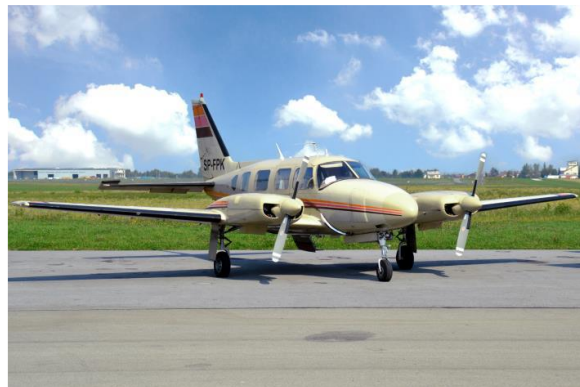
Figure 6. Piper Navajo PA-31, modified for LiDAR scanning
