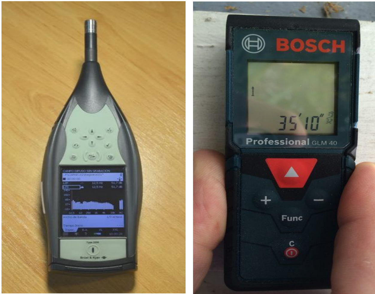
Fig. 6 Equipment used in experiments sound meter and laser measure tool
