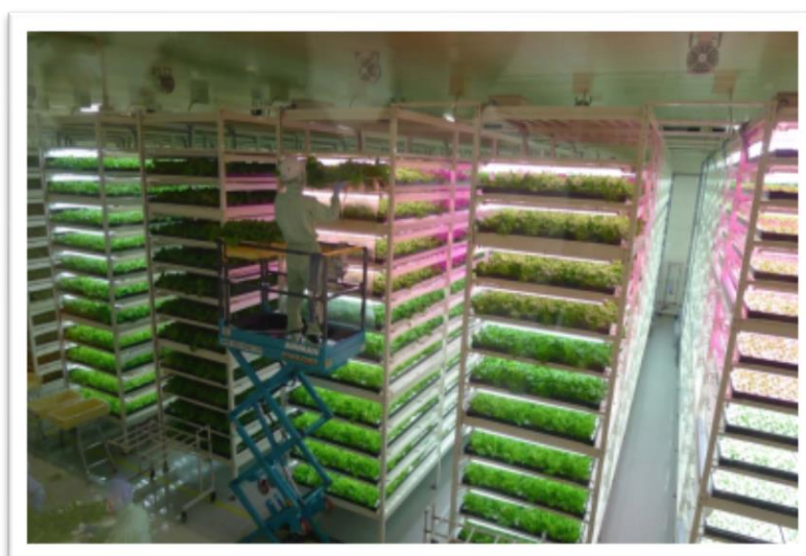
Fig. 29: Fully automated closed-door chamber for the industrial production of "ready-to-eat" seedlings and / or vegetables
