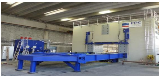
Figure 4.4.1.3-1 Equipment with capacity of vertical load of 50000 kN
