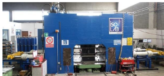
Figure 4.4.1.3-2 Equipment with capacity of vertical load of 70000 kN
