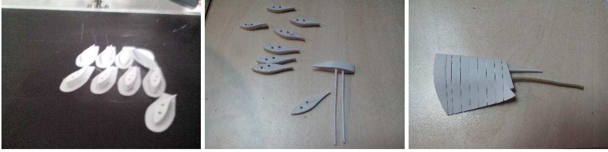
Figure 2.5 – The process of 3D printing of the components of the rotors blades
