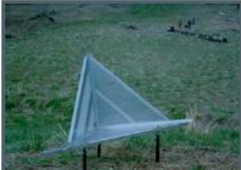
Figure 4. Corner reflector for radar signal
