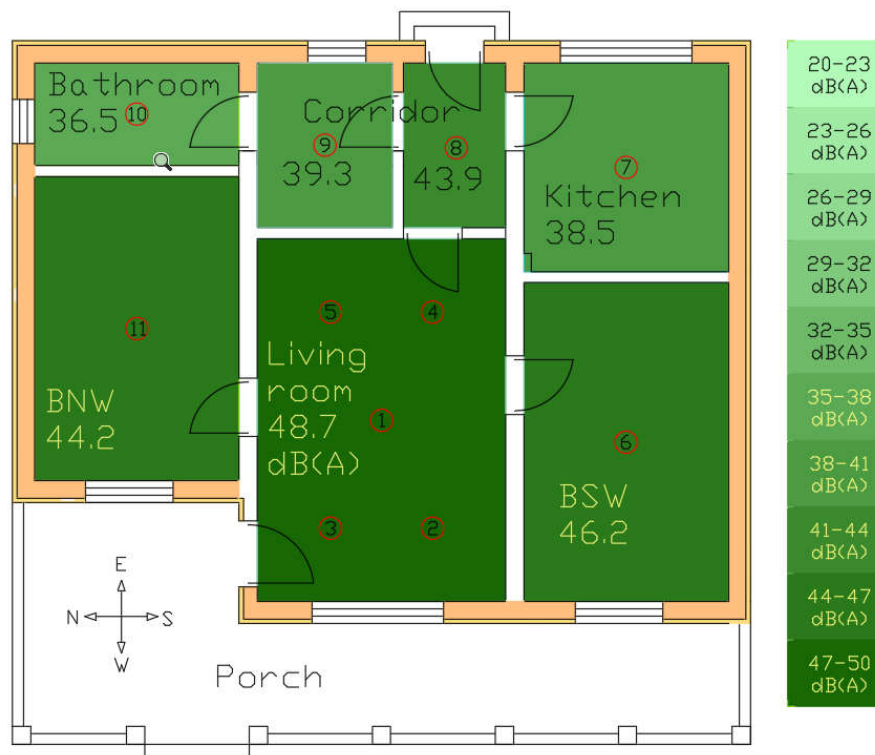
Fig. 11. Sound pressure level distribution during maximum ventilation rate (37,32 m 3 /h).
