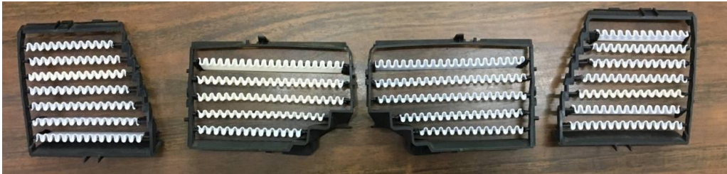
Figure 7: Air diffusers with lobed ailerons before painting
