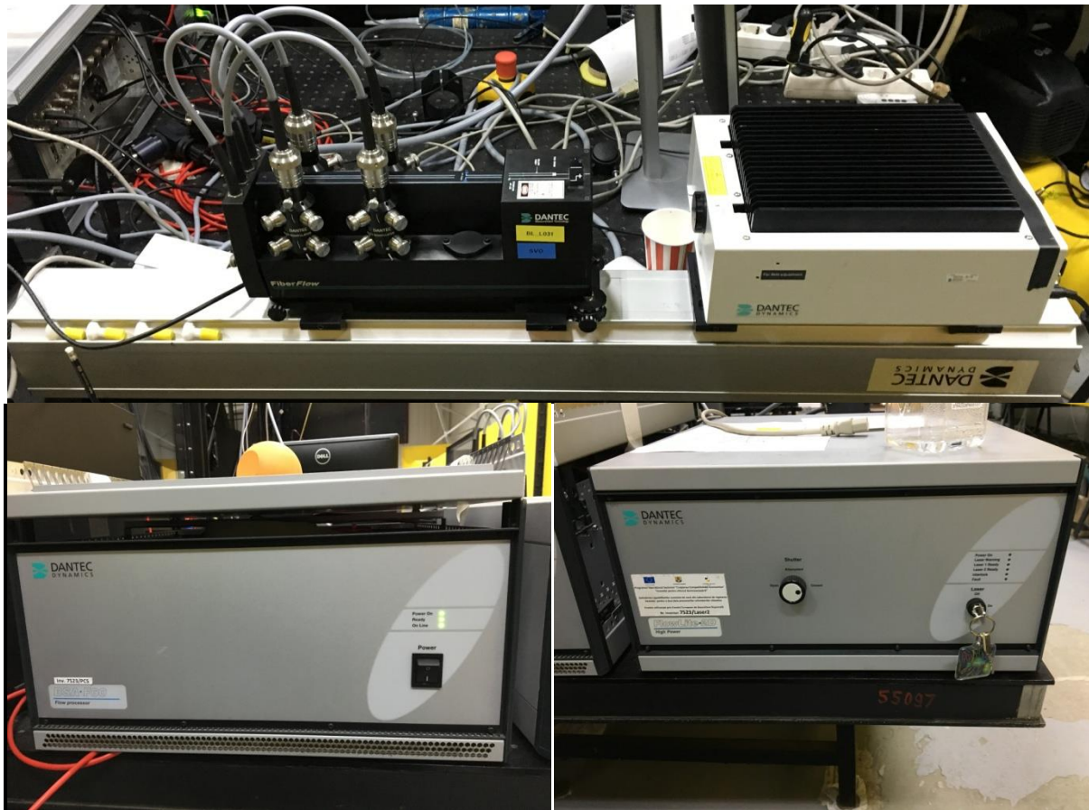
Figure 43. 3D-LDA measuremet system used
