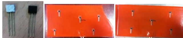
Figure 16. Temperature sensors stick on heating elements
