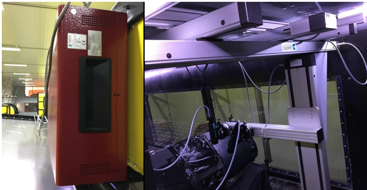
Figure 43. 3D-LDA measuremet system used
