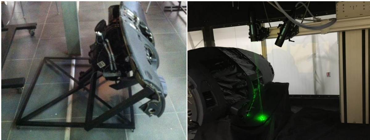
Figure 34. laser beams passing through pin hole
