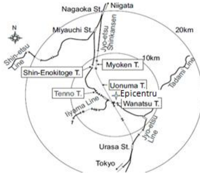
Fig.3.11. Distribution of severely damaged tunnels upon the Niigataken-Chuetsu earthquake.
