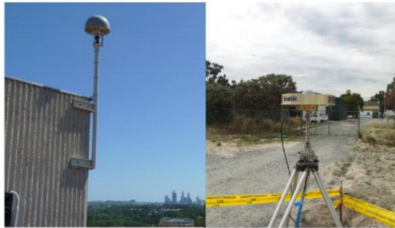
Fig.4.11. Zero-Baseline Receiver used in Perth (2013-2014) for inter-system bias calibration (Robert Odolinski, IGNS 2015)
